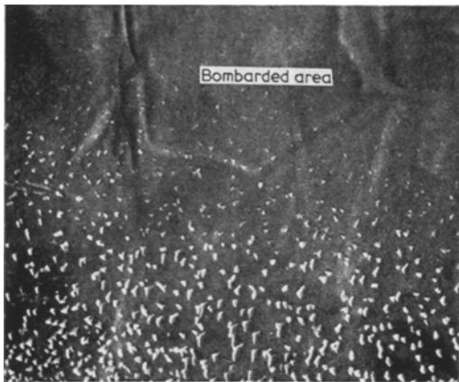
Figure 10 Bombardeed area boundary on iron surface, bombarded with 20 keV Ar + ions at \phi = 0^\circ for 30 min ( t = 900^\circ\text{C} ) \times 1000 .
